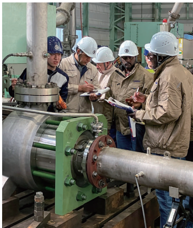
RO High Pressure Pumpの立会試験
