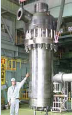
Boiler Circulating Pump KSK Coal Fired PP India, 6x600MW
