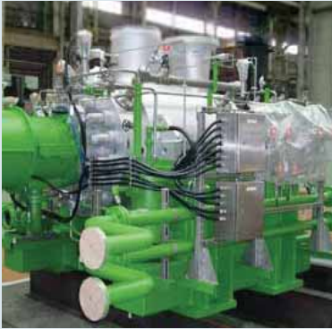
Barrel Type Boiler Feed Pump Cirebon Supercritical Coal Fired PP Indonesia, 1x660MW
