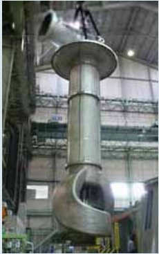
Hot Well Pump Polaris Geothermal PP Nicaragua, 1x72MW
