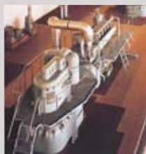
Pumping equipment for drainage station
