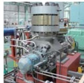
Ring section type boiler feed pump
