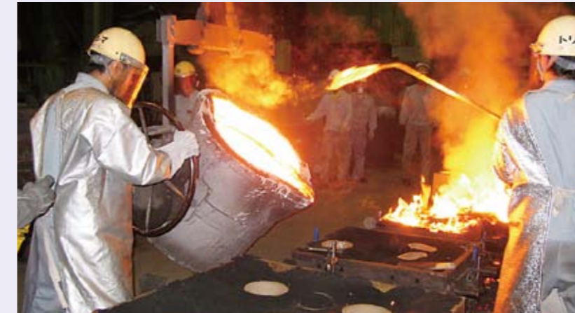
Pouring into small, middle-size mould
