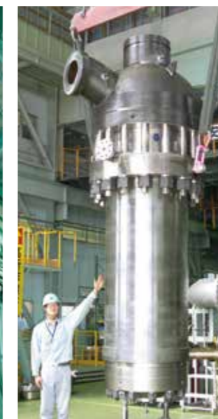
KSK Coal Fired Power Plant 6 x 660MW, India HLAV spherical casing boiler circulation pump
