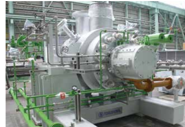
Chhabra Supercritical Coal Fired Power Plant 2 x 660MW, India MHB barrel type boiler feed pump [15MW drive, 50% duty]
