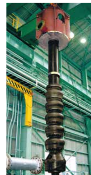
Altamira II Combined Cycle Power Plant 1 x 495MW, Mexico MMTV condensate pump
