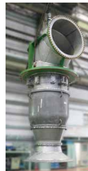
Vung Ang Coal Fired Power Plant 2 x 600MW, Vietnam SPV cooling water pump
