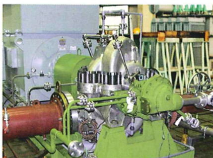
Hamma (Algeria), 2006 ;— MSH300/2 1072m 3 /h at 543m 2250kW
