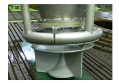
Pump with submersible motor
