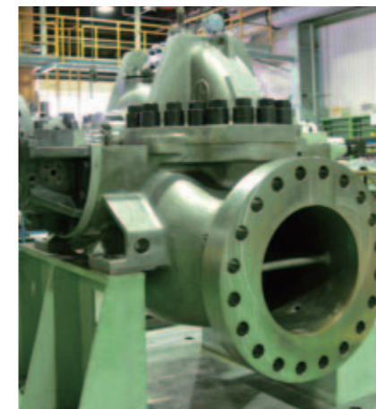
High-pressure pump for RO desalination in Saudi Arabia
