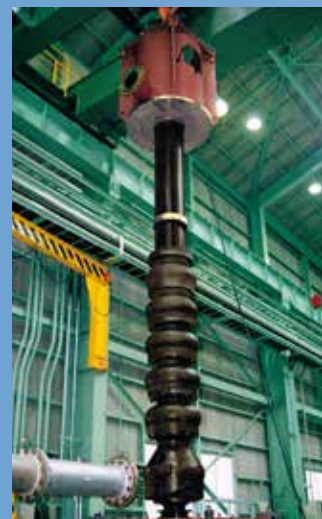
Condensate Pump Altamira II CCPP Mexico, 1x495MW
