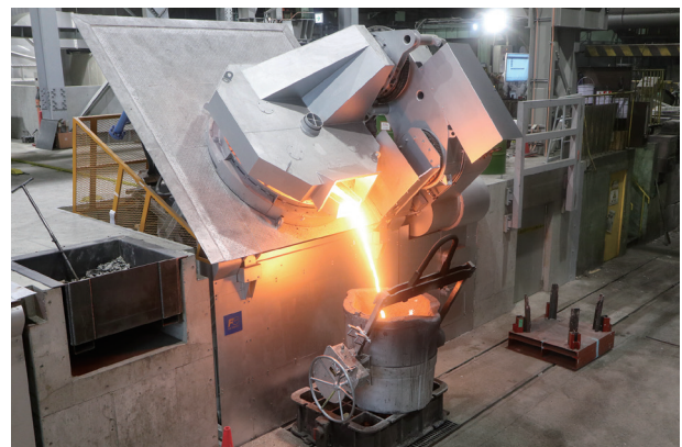
First molten metal produced in the new high-frequency electric furnace
