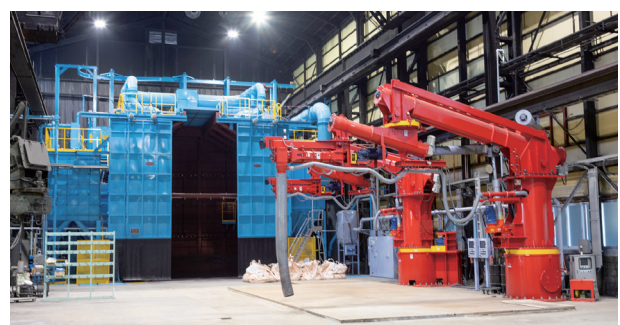
Updated shake-out machine (blue) and mixer (red)
