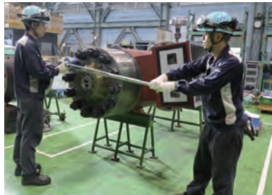
Assembly of specialized pump
