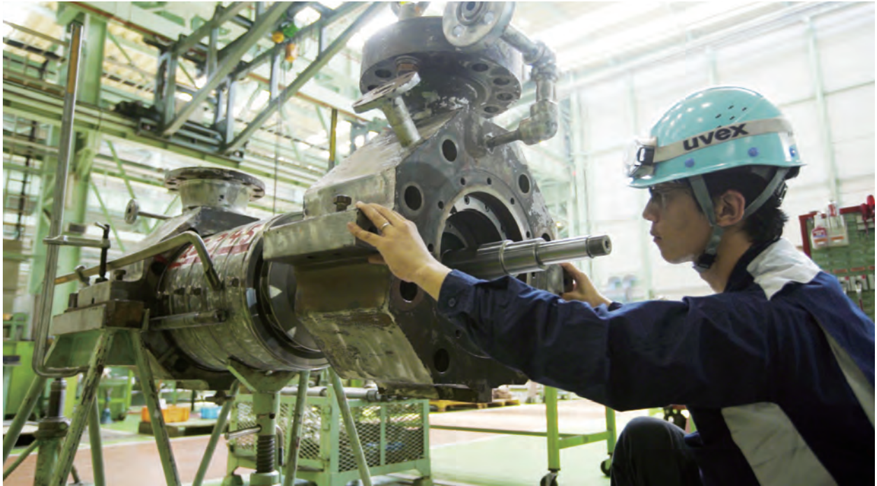
Maintenance of boiler feed pumps at Torishima's factory
