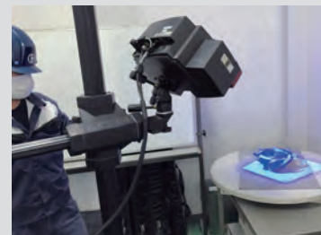
3D shape evaluation of impeller using ATOS
