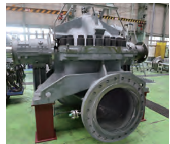
Long-distance pumps for transporting drinking water
