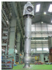
Seawater intake pumps
