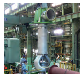
Hotwell pumps for geothermal power plants
