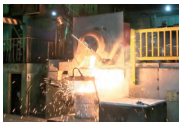
Melting and discharging of iron with electric furnace
