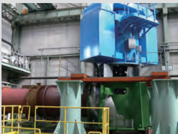
Performance test of large vertical pump
