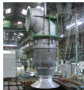
Water circulation pumps
