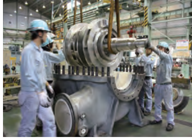
Assembly of large horizontal pump
