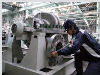
Dimensional inspection of high-pressure pump
