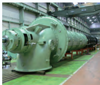
Stormwater drainage pumps for drainage pumping stations
