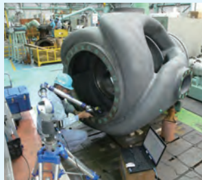
3D scanning of casings
