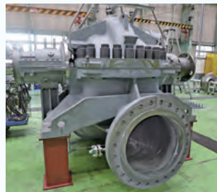
Long-distance pumps for transporting drinking water at desalination plants
