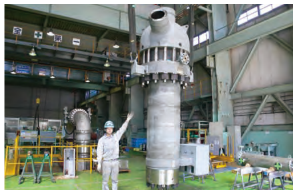
Boiler circulation pump
