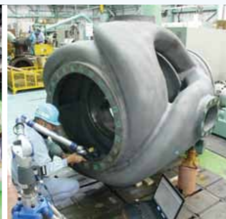
3D scanning of casing
