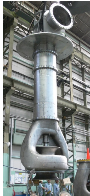
Brine circulation pump UAE
