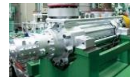
2015 Development of new boiler feed pump
