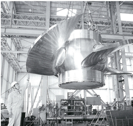
Adjustable vane propeller of 3600 \phi vertical axial-flow pump
