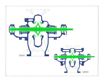
CDKS, CDKD, volute casing pumps with double flow impeller, are pumps of horizontal radially split casing with side covers.
