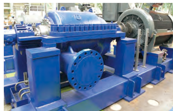
Reverse-osmosis high-pressure pump
