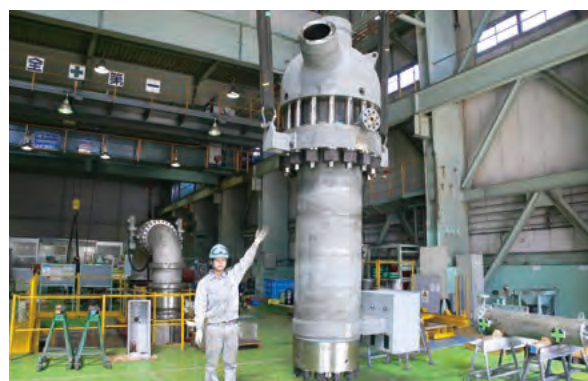
Boiler circulation pump
