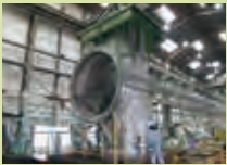
Circulation water pump for power plant
