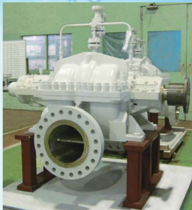
First-pass high-pressure pump delivered for the seawater desalination plant in Saudi Arabia in 2012
